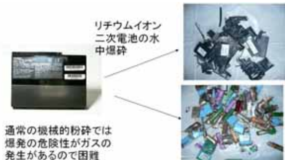
Photo 2 Separated lithium ion battery by underwater explosion.
